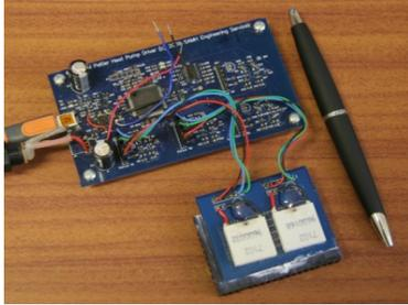
**Figure 1: Microcontroller and Peltier stimulators used in the experiments.**
